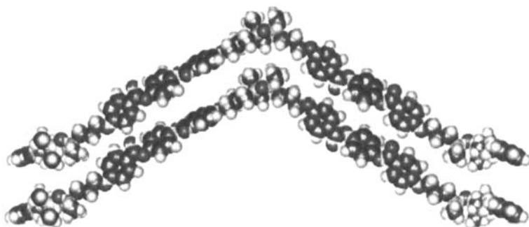
FIGURE 10 Geometric arrangement resulting from X-ray-measurement of the mechanically oriented fibre. (The polymer strand is perpendicular to the fibre direction). (See Color Plate II).
